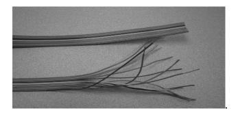
Description: Each conductor is stranded T.C. with extruded PVC insulation, bonded together to form a flat ribbon cable. Conductors separate easily for clean terminations with standard wire connectors, jacks and pins.
