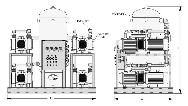
NOTE: Modular bases are available to facilitate access through 36" door openings
