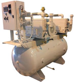
Each vacuum pump is supplied with an inlet check valve, inlet isolation valve, built-in anti-suck-back valve, inlet filter screen, oil sight gauge, oil drain valve, exhaust pressure gauge, high discharge temperature switch, inlet and discharge flexible connectors and a shut-off cock for gauge and vacuum switches.
